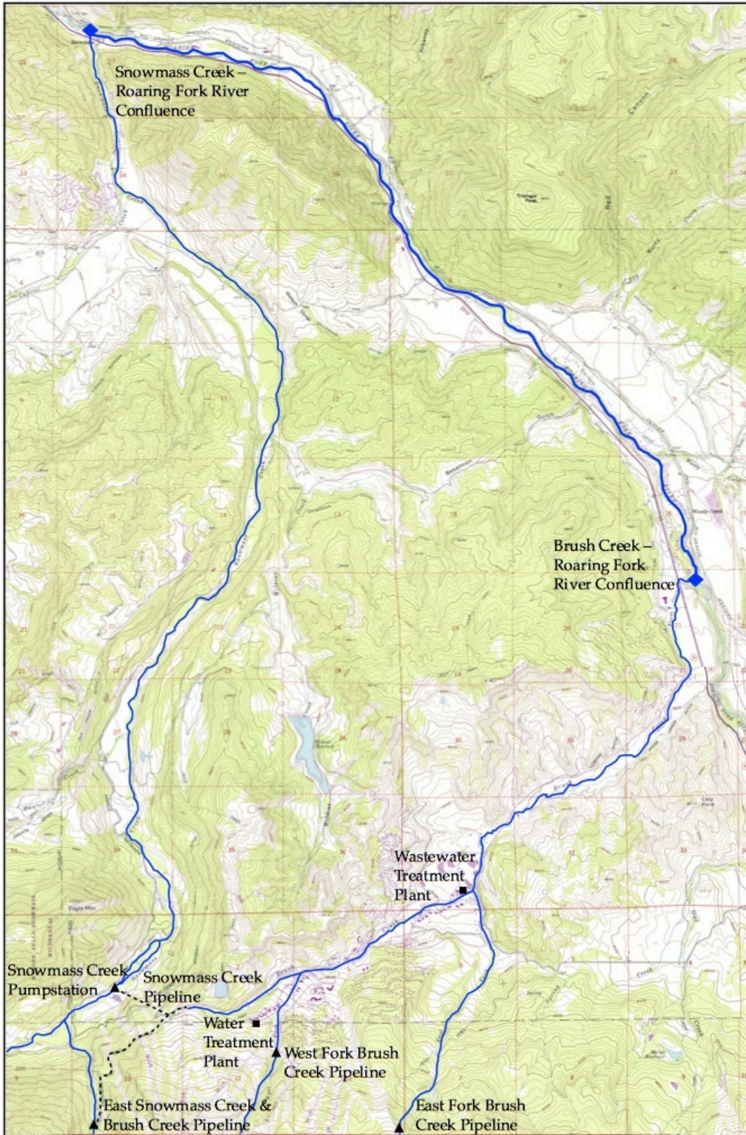
Figure 5. East Snowmass and Snowmass creeks are the primary sources of water for the Snowmass Water & Sanitation District's water collection system, due to the impaired water quality and limited physical supplies in the Brush Creek drainage. Return flows from the district's transbasin diversions are discharged and released into lower Brush Creek, where they eventually rejoin the source waters at the confluence of Snowmass Creek and the Roaring Fork River. (USGS, adapted from W.W. Wheeler, 2006)
