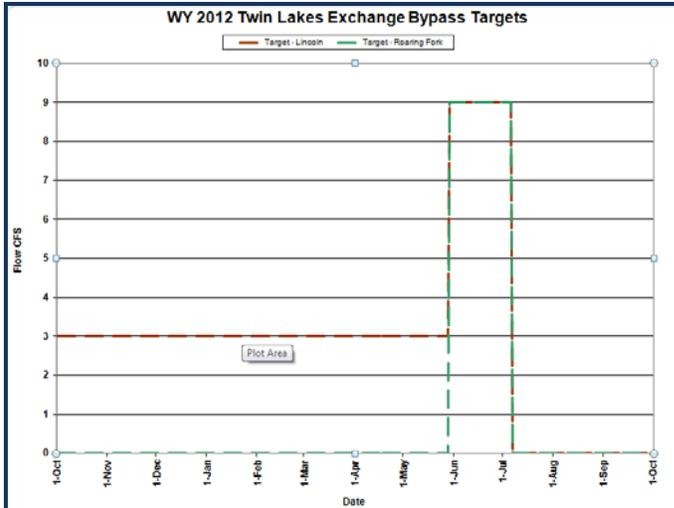
However, the V-notch weir on the Upper Roaring Fork River that measures flow below the IPTDS is limited in capacity to 4-5 cfs. A new gage or measuring device in this area would allow bypassing equal amounts in the future. To reflect this limitation starting on May 29, 2012 Lincoln Creek started bypassing 13 cfs, and the Roaring Fork at Lost Man bypassed 3 cfs.
