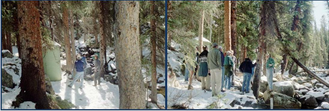
Roaring Fork above Lost Man Creek near Aspen stream flow gage (Oct, 2005). Ice and snow in the winter and the rocky substrate hinder accurate, year-round stream flow readings.
