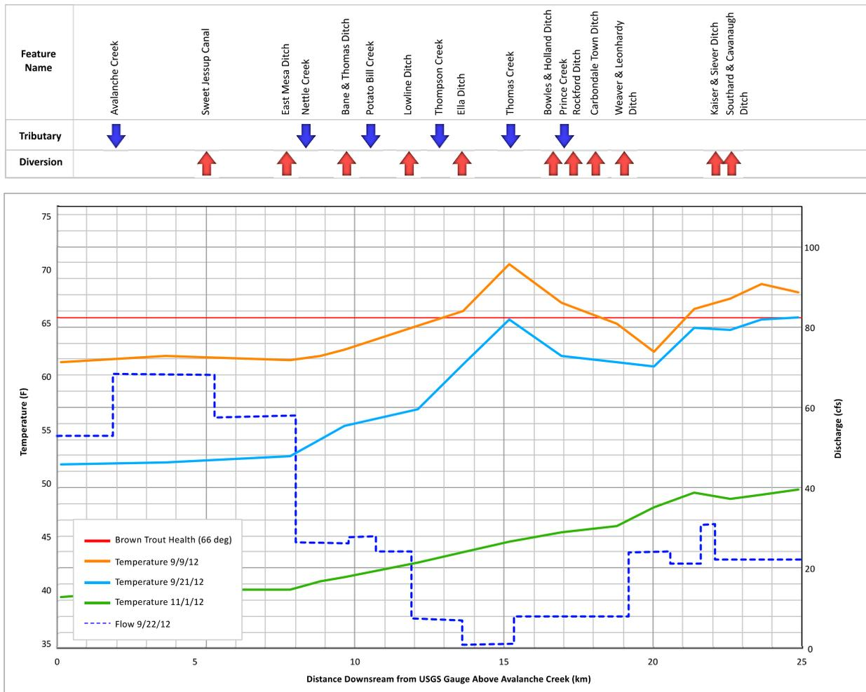
Figure 12. Observed temperatures on the Crystal River. Temperatures rise rapidly as flow decreases, peaking in the area near Thomas Road.
