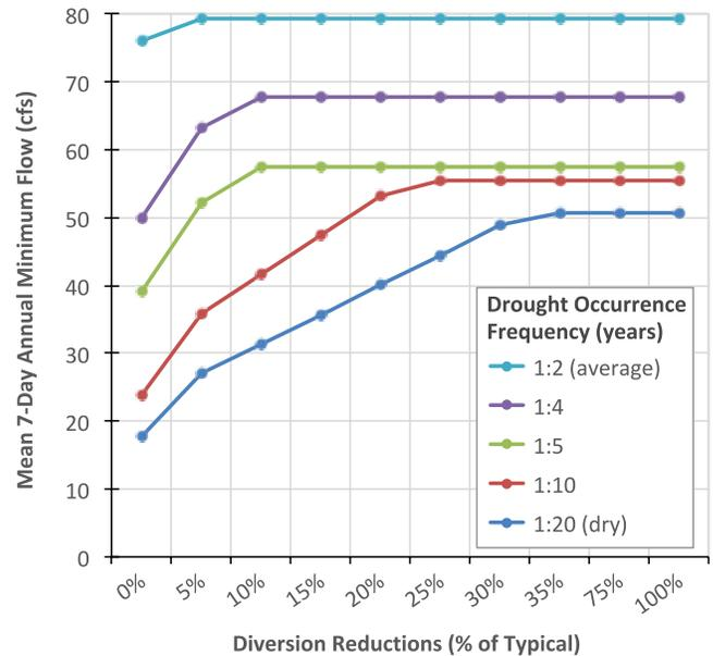
Figure 4-2: Changes in 7Q at the Thomas Road Bridge as a function of diversion reductions. Diversion reduction may be achieved through Non-Diversion Agreements, conservation gains resulting from ditch lining or sprinkler irrigation, or a combination of the two. Upper inflection points on the 7Q curves indicate a transition to optimal hydrological regime behavior
