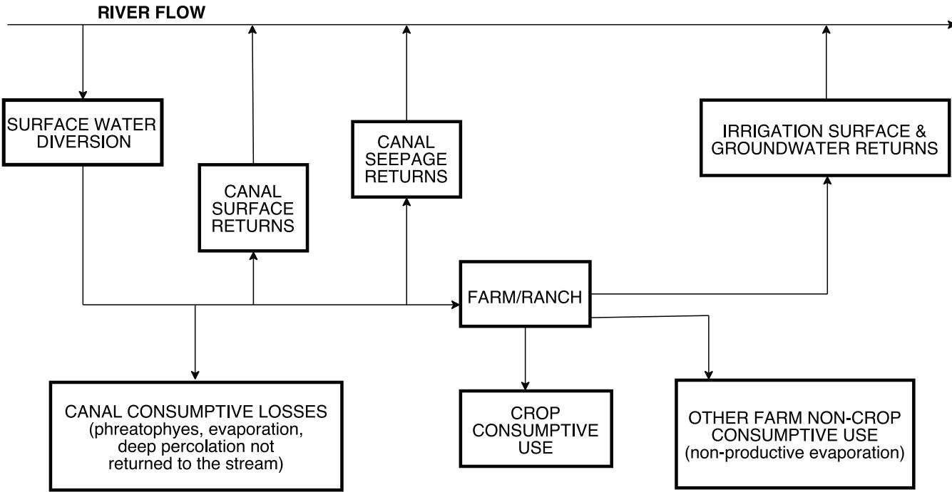
Figure 3-4: Irrigation system schematic indicating the various pathways water travels along between a point of diversion and a point of use.<sup>10</sup>
