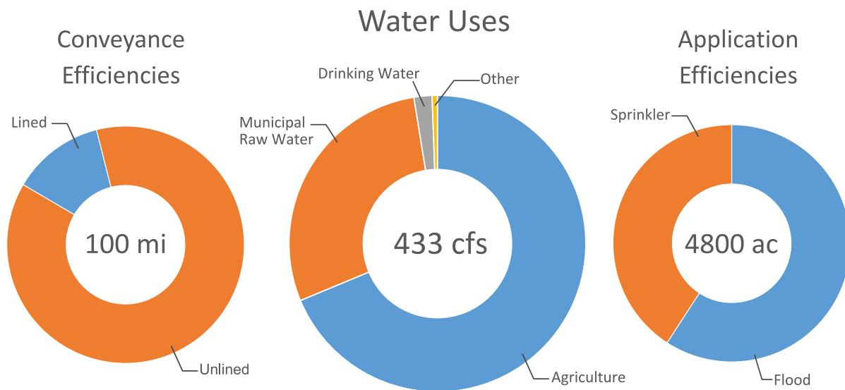
Figure 3-1: Summary of water uses and supporting infrastructure on the Crystal River and its tributaries. 433 cfs of surface water diversions are conveyed along approximately 100 miles of ditch and pipe to support municipal uses and about 4800 acres of irrigated land
