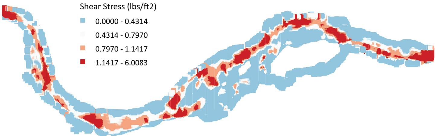
Figure 2-6: 2-dimensional hydraulic modeling simulated streambed shear stress conditions across a range of streamflows and allowed for assessment of sediment mobilization potential
