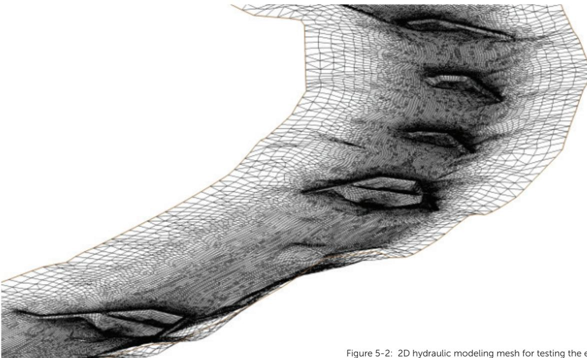
Figure 5-2: 2D hydraulic modeling mesh for testing the effectiveness of artificial habitat enhancement structures on the Crystal River
