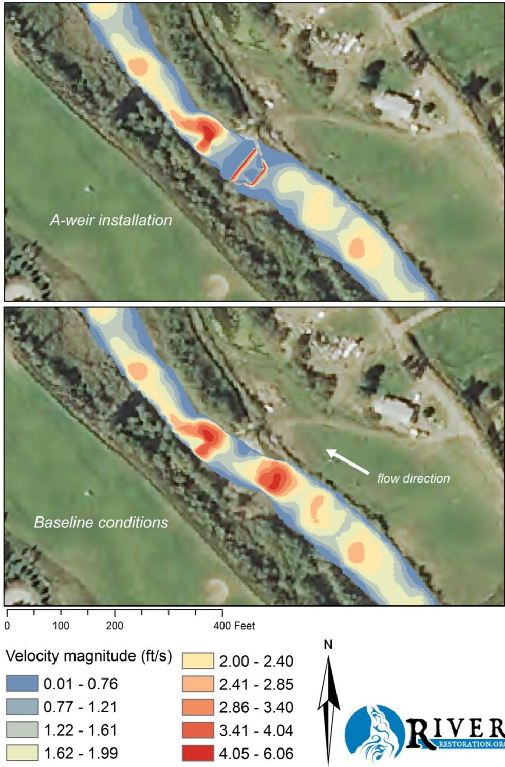
**Figure 13.** A-weir structure and existing conditions results, 100 cfs
