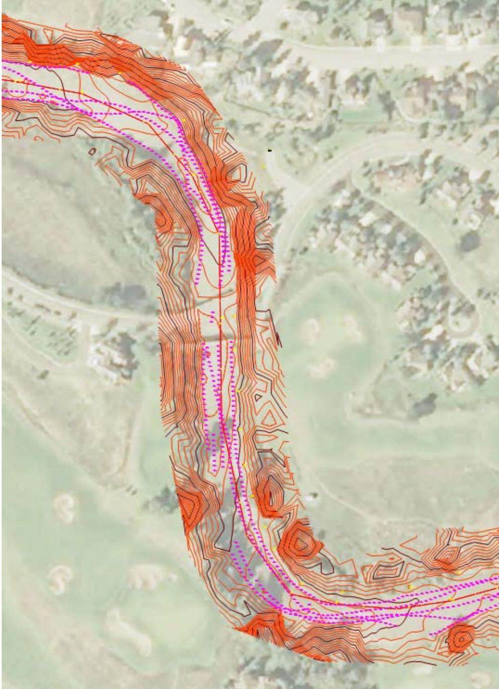
**Figure 3.** Surface created from survey points, vicinity of Crystal Bridge Rd. Red contours at 1 ft, black at 5 ft; flow direction upwards
