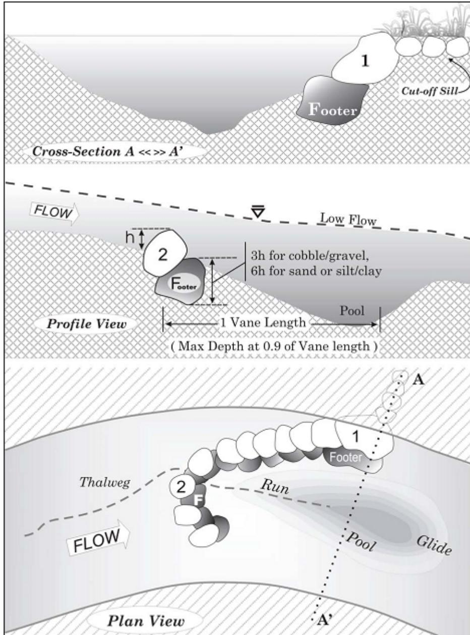
Figure 18. J-hook schematic from Rosgen (2006)
