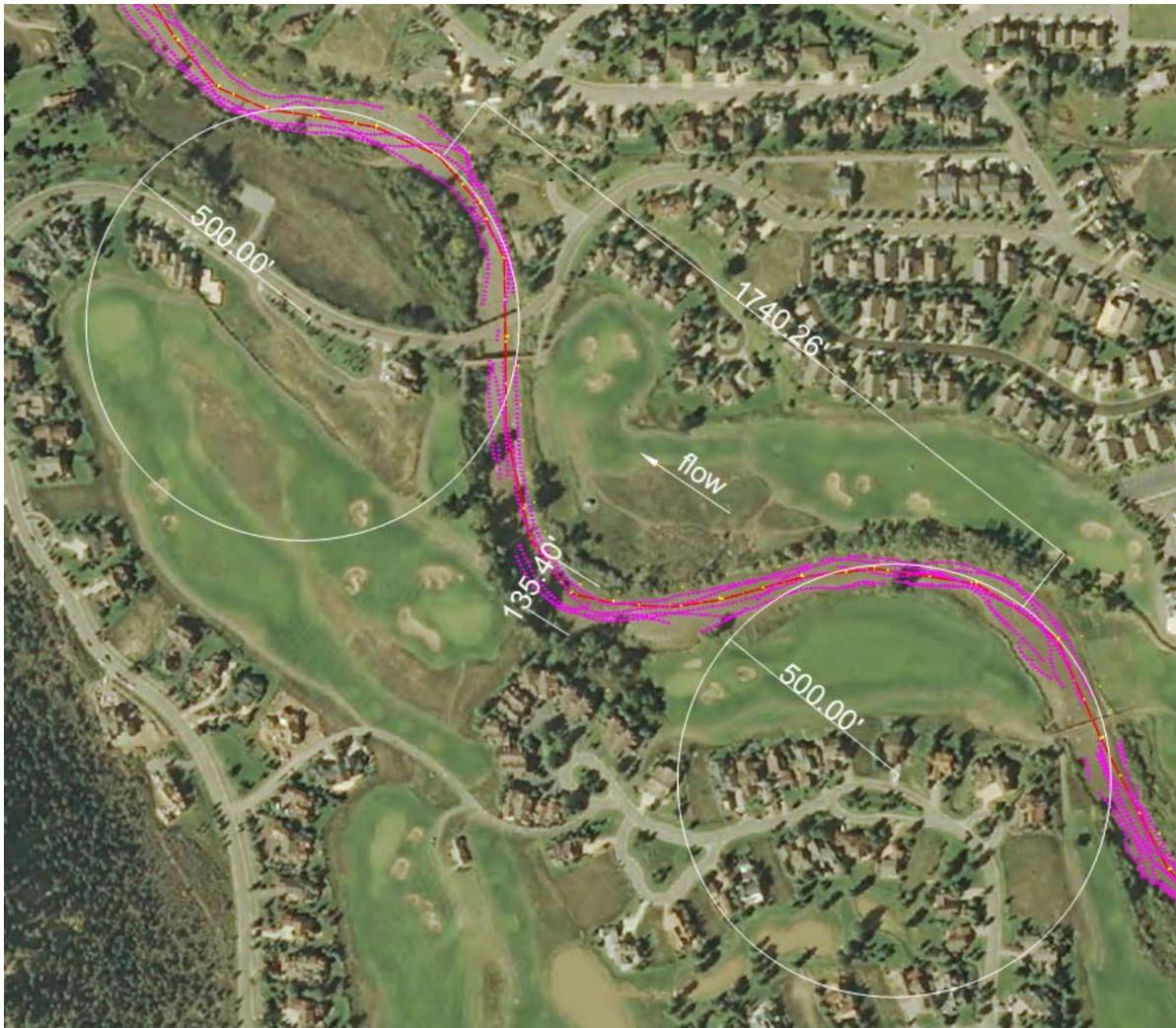
**Figure 2.** Crystal Bridge Rd vicinity, meander length, radius of curvature, and top width. Instream survey points and alignment illustrated
