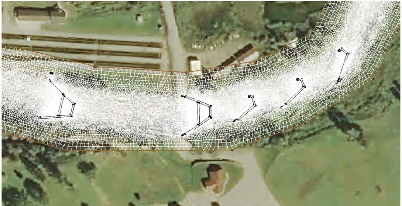
**Figure 21.** Planimetric view of conceptual restoration design computational mesh, near Mt Sopris Ranch Rd Bridge, flow direction to left
