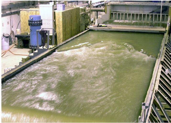
**Figure 9.** Laboratory A-weir under bankfull testing conditions
