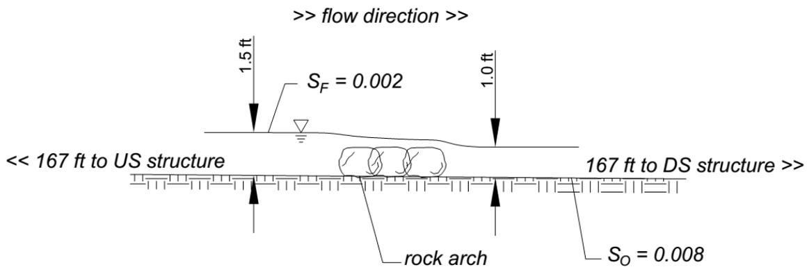
**Figure 15.** Profile view of LFHC design at rock-arch structure
