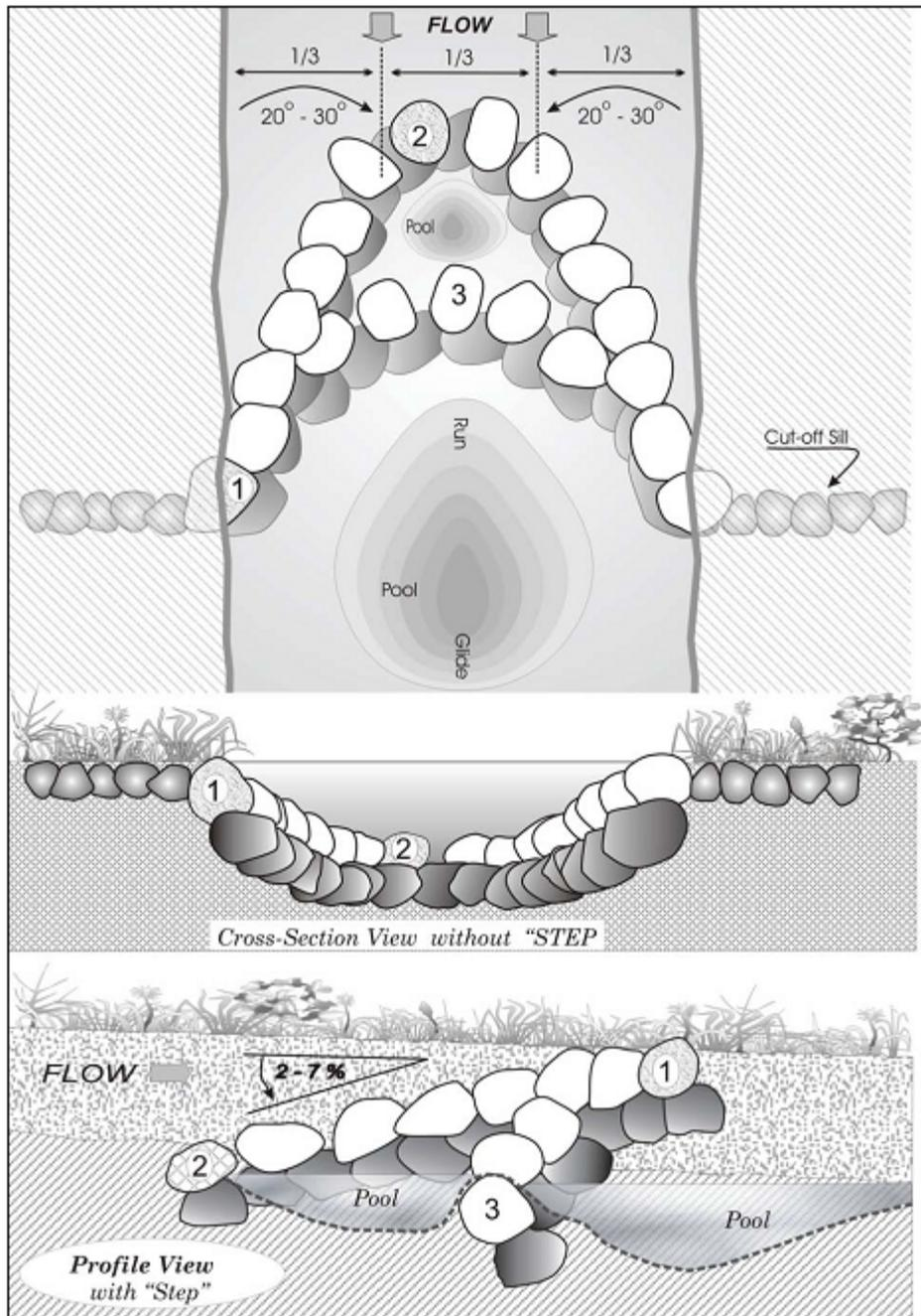
**Figure 8.** A-weir schematic (Rosgen, 2006)
