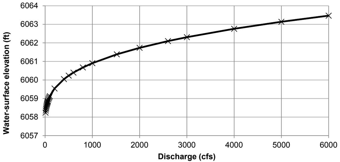
**Figure 6.** Existing conditions model downstream boundary rating curve
