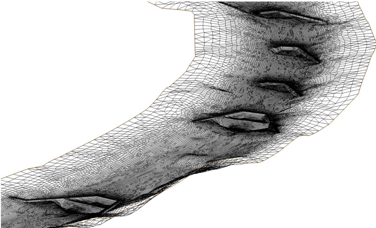
**Figure 22.** Perspective view of Wildland Hydrology (2014) conceptual restoration design computational mesh, near Mt Sopris Ranch Rd Bridge
