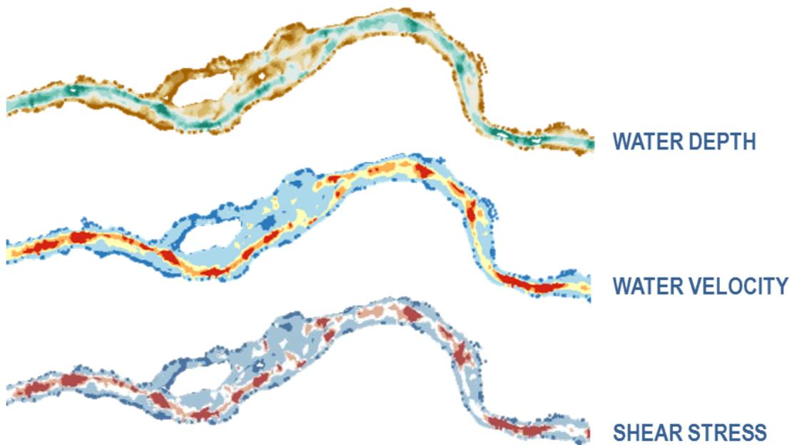
**Figure 14. Simulation outputs from 2-dimensional modeling for hydraulic parameters including water depth, water velocity and shear stress.**
