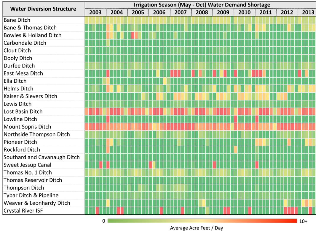
Figure 9. Diversion shortages under existing conditions predicted by the EcoDSS.
