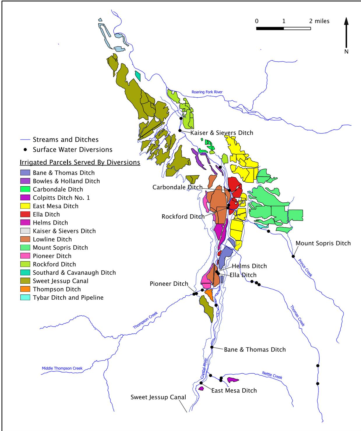
Figure 10. Map of irrigated parcels and associated diversion structures on the lower Crystal River
