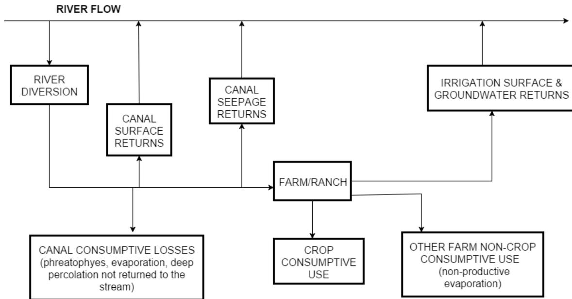
**Figure 8. Irrigation system schematic demonstrating the paths water flows along before being consumed by crops or returning to the river. Adapted from Colorado Agricultural Water Alliance (2008).**
