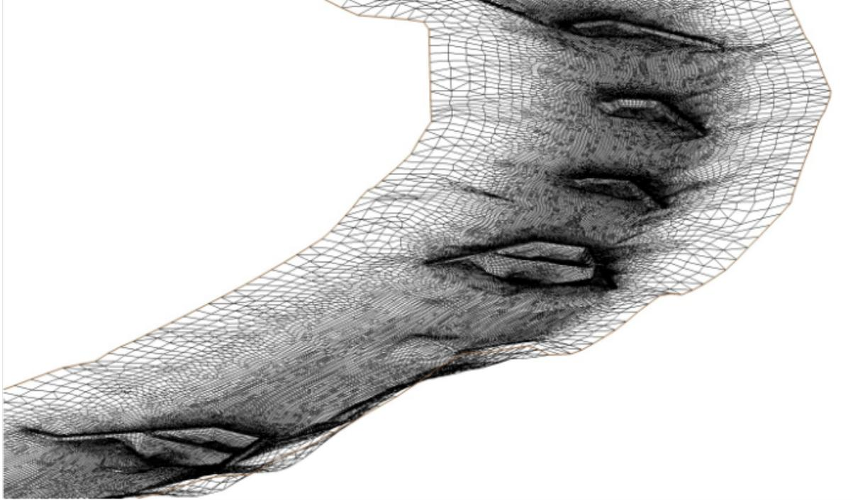
**Figure 13. Example of the hydraulic modeling mesh utilized to test the second-order impacts of management and structural alteration on the Crystal River.**
