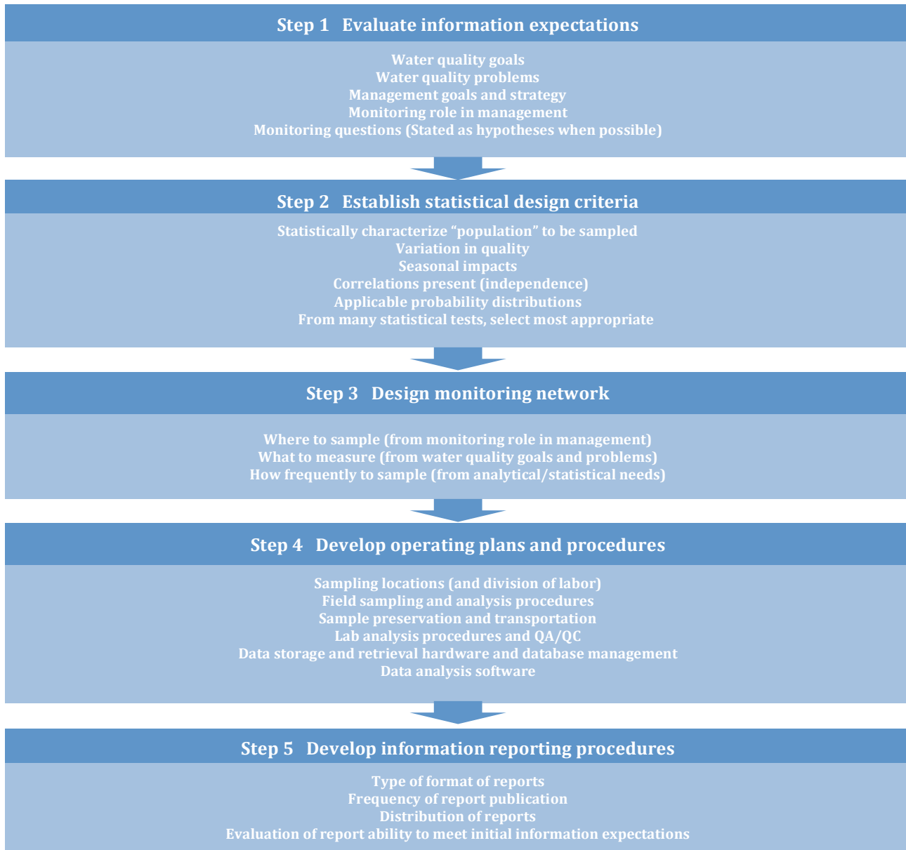
Example design process for water quality monitoring plans. Adapted from Ward et al. (1986).
