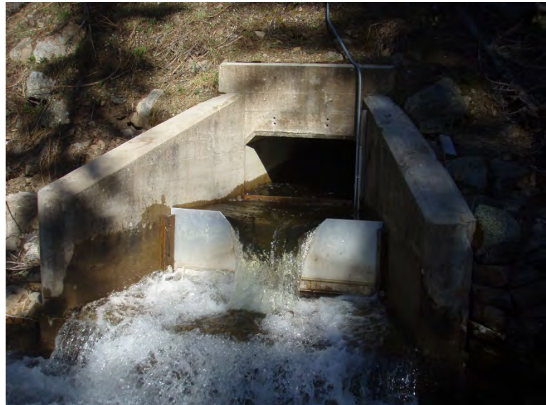
This V-notch weir is the current USGS-run gage setup on the upper Roaring Fork at Lost Man. Only able to measure flows below 5 cfs, it does not operate in the winter due to icing.
