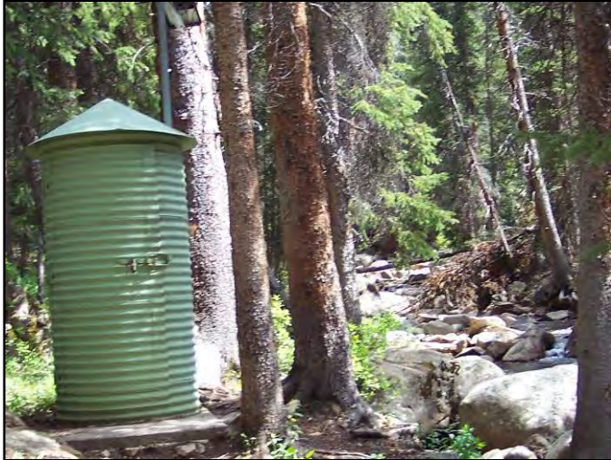
Figure 4. CDWR Roaring Fork above Lost Man Creek near Aspen stream flow gage, July 8, 2005. Ice and snow in the winter and the rocky substrate hinder accurate, year-round stream flow readings.
